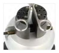
Mounting via retaining pins
