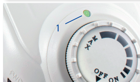
Fig. 7.3 LED control indicator
