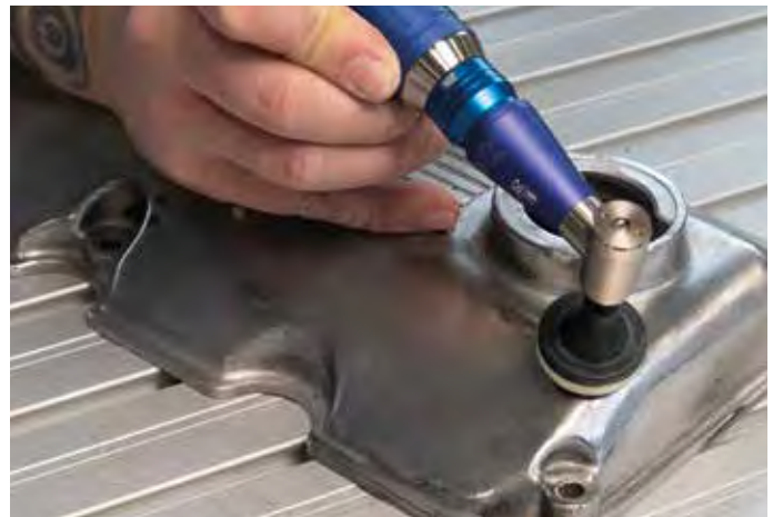
Aluminium polishing with angle-handpiece and felt
