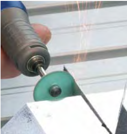
Cool cut with a ceramic fibre cut-off disc
