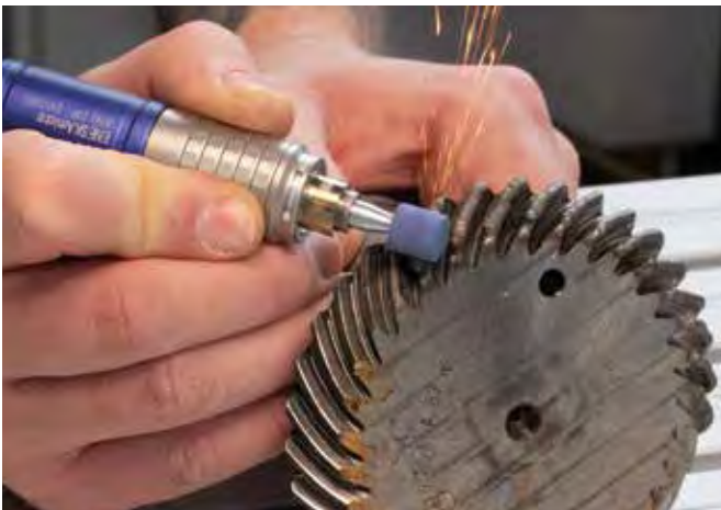
Welding seam with Blue Stones grinding
