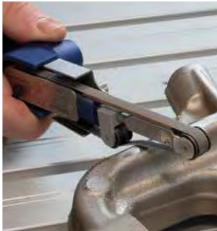
Convex shapes - belt grinder and grinding belts
