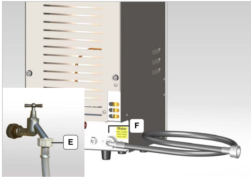
Figure 4.4.3: Connected water hose
