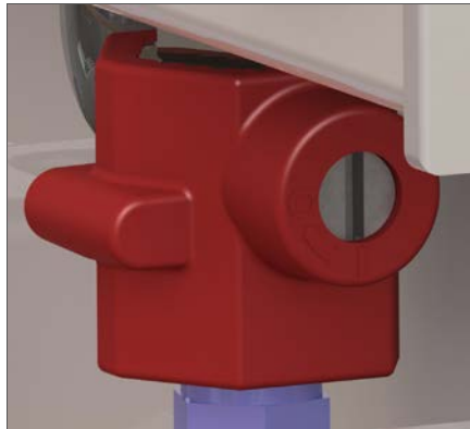
Figure 7.4.5.1.3: Ball valve Open
