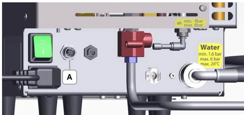
Figure 4.2.1.1: Connection for the Foot Switch (Rear panel)
