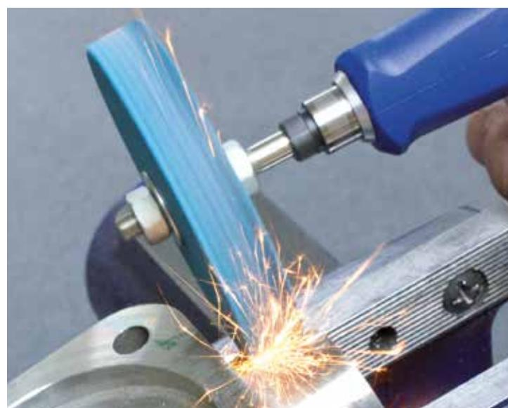
removing of milling traces from 1.2379
