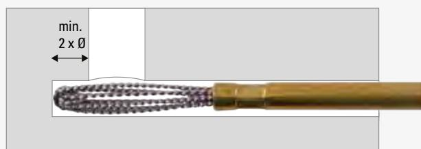
3. **Wire, knotted:** for transverse holes at the bottom of the blind hole. For removing very heavy burrs.
