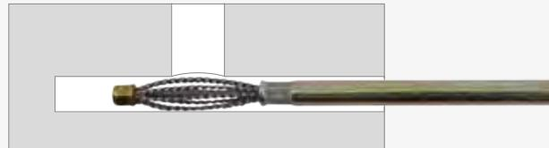
2. **Wire, crossed:** for transverse holes and end face processing in addition to non-concentric holes.
