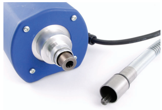
Figure 7.2 Connection of motor and shaft (here: Quick-Change-System)
