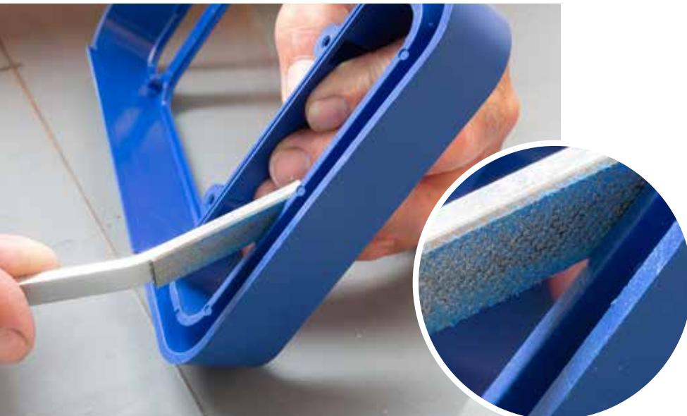
reworking of a carbide cutting edge with metal bond
